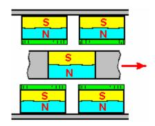
To increase the power of the output shaft further again, additional sets of magnets and coils can be added as shown here:
