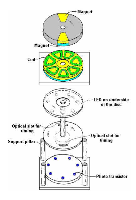
This construction is relatively simple and yet the operation is powerful. The power is provided by three magnets, shown shaded in blue and yellow. The lower magnet is in the form of a disc with the poles arranged on the large, circular, flat faces. This is the stator magnet which does not move. Positioned above it is a disc made of non-magnetic material (shaded in grey) and which has two magnets embedded in it. This disc is the rotor and is attached to the central vertical shaft.
