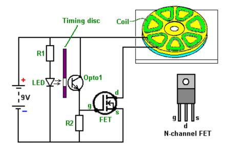
Just five components are used. The current through the coil is controlled by a transistor. In this case it is a Field-Effect Transistor usually called a "FET". The most common type of FET is used, namely an "N-channel" FET which is the rough equivalent to an NPN transistor as described in Chapter 12. A FET of this type is switched off when the voltage on it's "gate" (marked "g" in the diagram) is 2.5 volts or lower. It is switched on when the voltage on it's gate is 4.5 volts or more.
