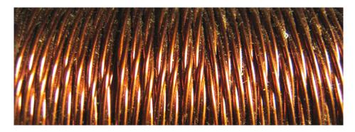
This completed coil now contains three separate coils in very close proximity to each other and that arrangement is excellent when one coil is powered up, for inducing energy in the other two coils. This winding now contains coils 1,2 and 3 of the circuit diagram. There is no need to concern yourself with marking the ends of each strand of wire as a simple ohmmeter will tell you which two ends have a winding between them.
