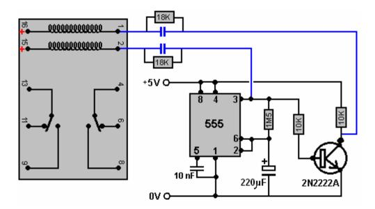
The capacitors shown in blue are chosen to operate the actual physical relay which is used in the circuit. They give the relay a brief switching pulse every five minutes or so. The 18K resistors across the capacitors are to bleed off the capacitor charge during the five minutes when the timer is in it alternative state.
