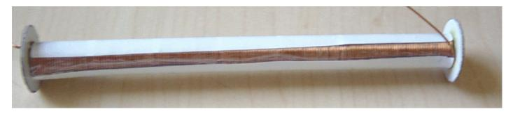
You now have a perfectly wound first layer. Before starting the second layer, cut the next strip of paper, measuring 40 mm wide. Stick a strip of Selotape along the length of the paper, again, with half of the width of the Selotape overlapping the paper and set it aside. Wind the next layer in exactly the same way, finishing by sticking and securing the paper around the core with its two layers of wire.
