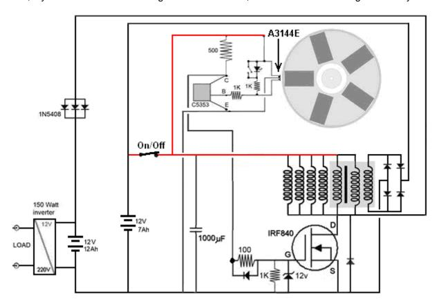
Here, the battery which powers the inverter which supplies the load is increased in capacity and while the developer used two of his 7 Amp-Hour batteries, you can use a standard 12-volt 12 Amp-Hour battery intended for a mobility scooter. All but one of the coils is used to supply current to the output
