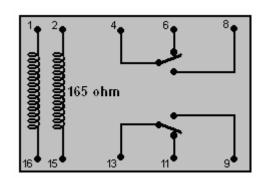
This is the electronic version of a mechanical two-pole switch. A brief pulse of current between pins 1 and 16 locks the switch in one position and later, a pulse of current between pins 2 and 15 locks it in the other position. The current drain on the circuit would be almost zero.
