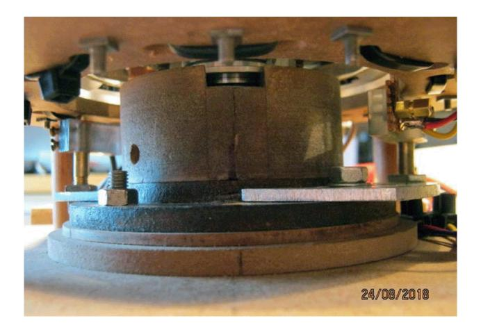
It is important to understand that while the 110 mm diameter rotor has five magnets located at even intervals around it's circumference, there are now ten coils on the surrounding stator, and there are now ten pulses per revolution. These pulses are powerful and when the current is cut off, each chain of five coils generates 600 volt spikes (although that can reach 900 volts on occasions).
