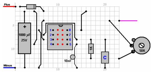
The capacitor "C" will be about 10 nF and the variable resistor can be 47K or 50K linear or a higher value could be used.
