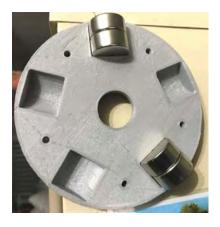
This 3D-printed rotor is made in two halves which are then bolted together.
