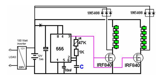
This arrangement allows for considerable alteration of the operating frequency by merely turning a knob. Experienced constructors will have their own preferred methods of construction, but we might choose to use a layout on an open board in order to make it easy to see what is happening and to give good cooling during the development stage, perhaps something like this:
