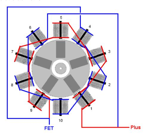
All ten coils are pulsed at the same instant and that instant is arranged to happen when a rotor magnet is between the two opposing coils. One coil pushes the magnet away and the other coil pulls that same magnet towards itself. This is very effective with the rotor spinning so fast that the developer describes it as being "scary" and he has to clamp it to the workbench because of the power being generated.
