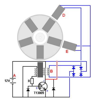
Coils "B", "D" and "E" are all triggered at the same time by three different magnets. The electrical energy produced in all three coils is passed to the four blue diodes to produce a DC power supply which is used to charge battery "A" which powers the circuit. That additional input to the drive battery and the addition of two more drive coils to the stator, makes the system operate securely as self-powered, maintaining the voltage of battery "A" indefinitely.
