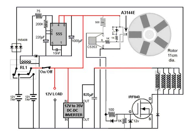
The developer stresses that the circuit operates in a non-intuitive way. First, the performance is somewhat reduced if the rotor spins faster which is something which is not at all obvious. Then it has been found that using ferrite magnets produces a better performance than using the stronger neodymium magnets. He sees it as the coil pulses being a mechanism for preventing 'cogging' or backward drag on the passing rotor magnets.
