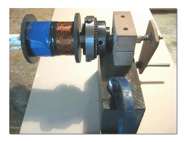
The three strands of wire which form coils "1", "2" and "3" are 0.7 mm diameter wire and they are twisted together to become a "Litz" wire before being wound into the coil "B". This produces a much thicker composite wire strand which is easy to wind accurately on to the spool. The winder shown above uses a chuck to grip the coil core for winding, but any simple winder will work well.
