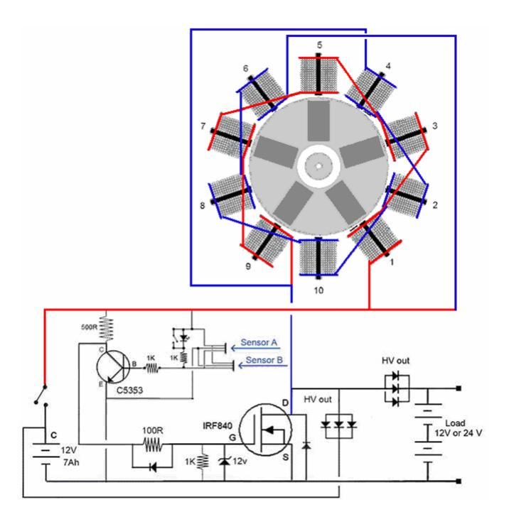
If we want to reproduce this performance without the rotor and it's magnets, then we need to apply 12-volt pulses to those two chains of coils 417 times every second. That may sound difficult if you are not familiar with electronics, but in actual fact, it is a very simple task and 417 Hz is very slow operation for an electronic circuit as they could easily generate 3,000,000 pulses per second.
