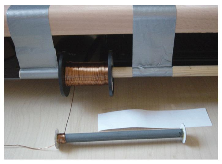
When the far end of the spool is reached, stick the piece of paper to the layer of turns using the Selotape already on the paper, bend the paper round the layer of winds and pull it tight using other
