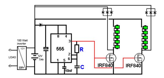
The resistor "R" and the capacitor "C" control the frequency of the pulsing and the result is very good. However, as the developer has powered both coil chains of his rotor circuit from a single transistor (although they generate at least 600V feedback pulses), he used just one transistor for his tests. He also likes to use his circuit which swaps over two drive batteries, one to provide current while the other one is recharging, but that is a minor matter.
