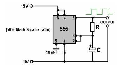
The capacitor used has to be high quality with very low leakage in order to get this waveform which is On for exactly the same length of time as it is Off. This is important if we want the two batteries to receive the same length of time powering the load as the time they receive being recharged.
