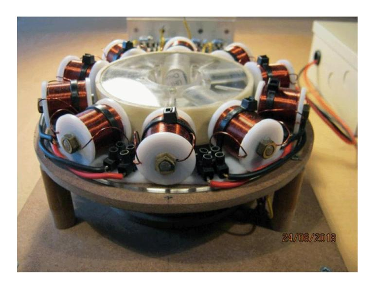
Remember that the coils are mounted on their own support ring and so can be handled as a single unit. This is very convenient.
