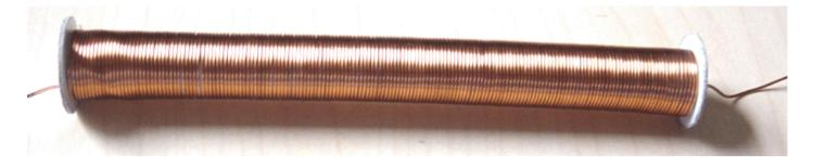
This generator can be built in thousands of variations, the main difference being the coils being used – the core material, the core length, the wire diameter, and the number of layers wound. You can, of course, start with one coil and see how your circuit performs, and later on, add one or more coils to boost the performance.
