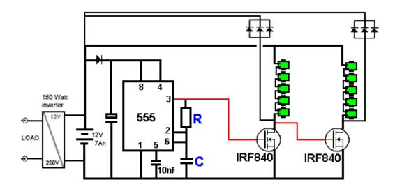
Then when the first transistor switches on, the second transistor switches off and vice versa. Doing that returns twice as many pulses per second to the drive battery without increasing the rate of pulsing of either of the coil chains. Remember also, that the transistors are powerful enough to drive several coil chains simultaneously, and each extra coil can be expected to increase the excess output power available.
