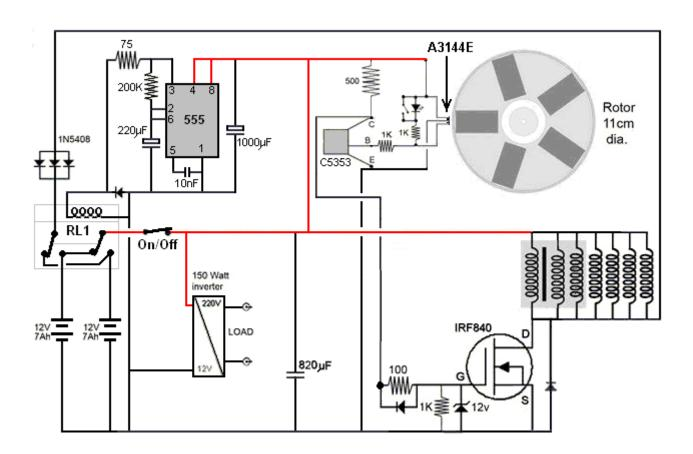
In this version of the circuit, a 12-volt non-latching relay is used. The relay normally draws 100 milliamps at 12 volts but a 75 ohm or a 100 ohm resistor in series lowers that current to about 60 milliamps. That current is only drawn for half the time as the relay is not powered up when the "normally closed" contacts are being used. The system powers itself very satisfactorily as before.
